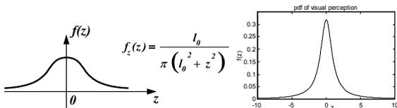
Fig. 3. Perception pdf along the  $z$  axis, i.e. parallel to the infinite plane in figure 1; the left figure is a sketch; the right one is a plot where  $l_o=1$
