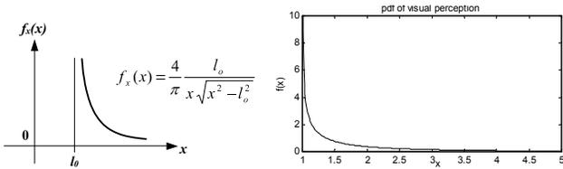
Fig. 2. Probability density function of the random variable representing the distance between eye and a location on the plane shown in figure 1; the left figure is a sketch; the right one is a plot where  $l_o=1$
