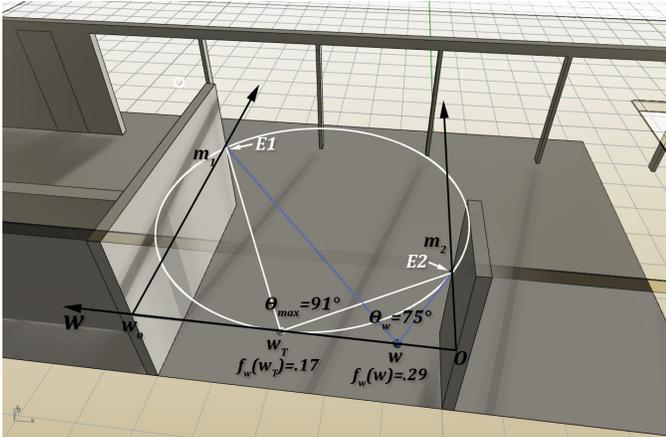
Fig. 7. One of the Pareto optimal designs, marked by an arrow in figure 8, where  $f_w(w) = 0.29/m$  and  $|w_T - w| = 1.64m$
