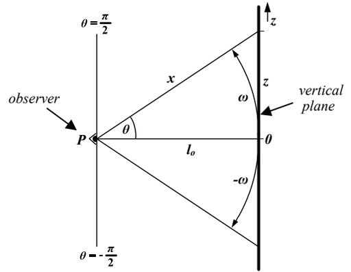
Fig. 1. The geometry of visual perception from a top view, where  $P$  represents the position of an observer, viewing a vertical plane at a distance  $l_o$  to the plane.
