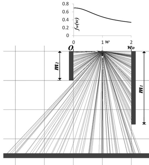
Fig. 6. Plot of  $f_w(w)$  where  $w_o=2m$ ,  $m_1=2.5m$ ,  $m_2=1m$  (upper), and the corresponding geometry (lower).
