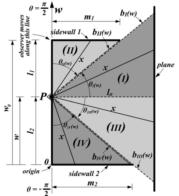
Fig. 4. Geometry involved in the computation of the probability density  $f_w(w)$  as to perception along the left most wall side, where the position of perception is denoted by  $P$ .
