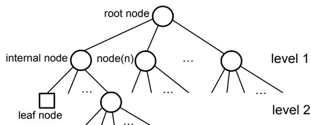
Fig. 1. The structure of a neural tree
