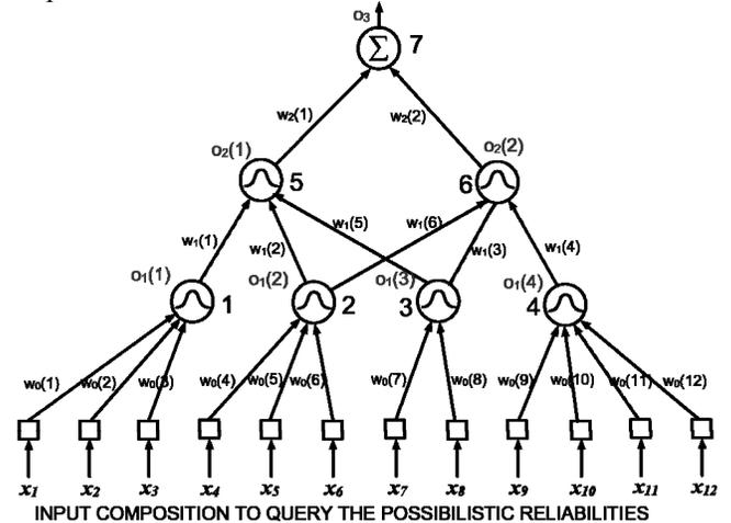
Fig. 5. The neural tree used in computer experiments for possibilistic reliability assessment
