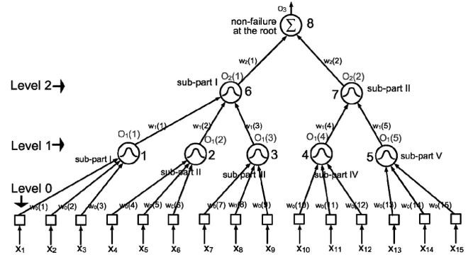
Fig. 4. An example of a neural tree employed for design
