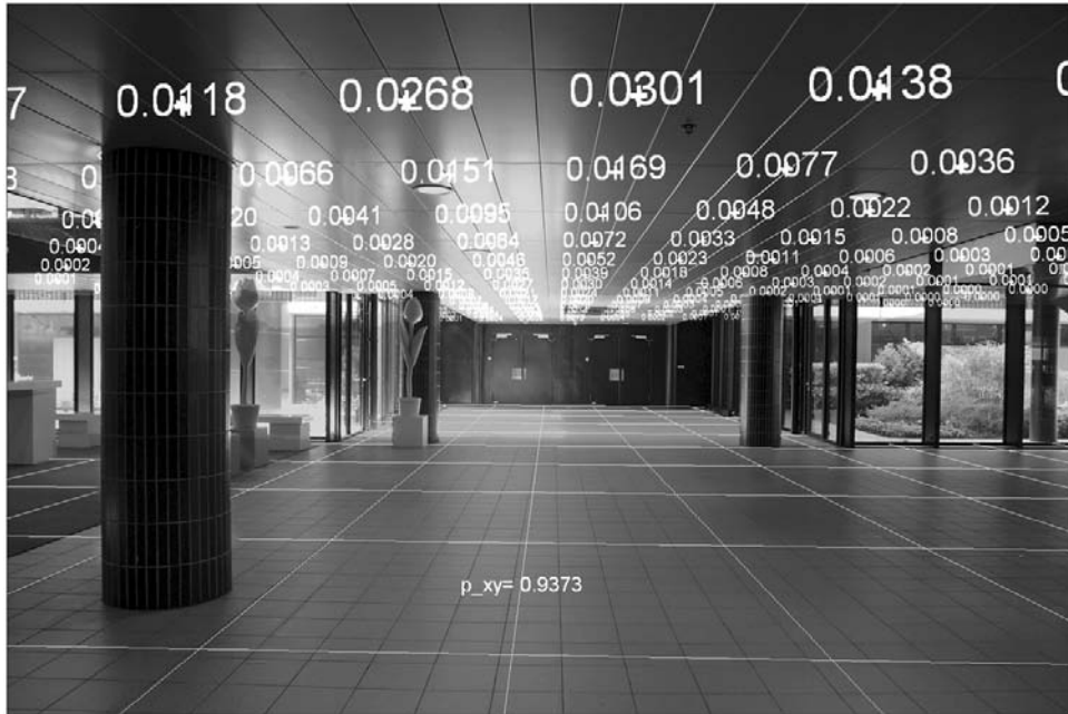
Figure 12 Space corresponding to the perception computation shown in Figure 9, where b = 22 m and l_b = 4.4 m, and the extent of the ceiling in x -direction (horizontal) is 18 m; the resulting degree of perception of the ceiling is P_{x,y} \cong 0.51
