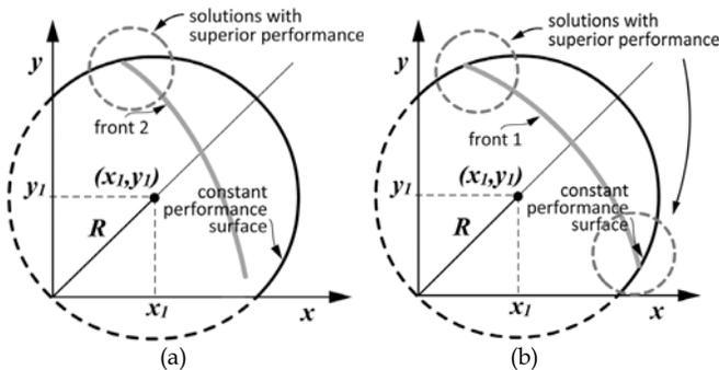
Figure 8. Dependence of the location of desirable solutions on the shape of Pareto front: front that is asymmetrical to the line passing from origine to the utopic point (a); symmetrical front (b)
